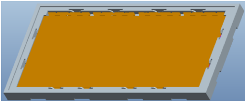
Put 1Pcs 4t EPE pad , ... , totally 8 pcs open cell and 9pcs EPE pad in one box,
