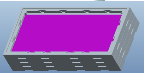
Put one paper pad on the pallet, Put totally 5 boxes and 1 cover, (5ea boxes per pallet)
