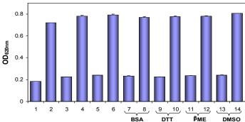
Phosphate assays in 96-well plate. 1. H<sub>2</sub>O, 2. Phosphate, 3. ATP in H<sub>2</sub>O, 4. ATP/Phosphate in H<sub>2</sub>O, 5, 7, 9, 11, 13: ATP in Assay Buffer with, where indicated, 0.5 mg/mL BSA, 1 mM DTT, 2 mM β-mercaptoethanol (βME) and 5% DMSO, 6, 8, 10, 12, 14: ATP/Phosphate in Assay Buffer. Phosphate and ATP were at 50  $\mu\text{M}$  and 1 mM, respectively. The assay is not affected by these components.
